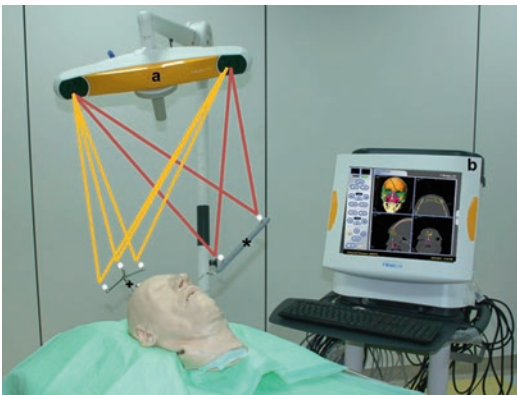
Fig. 5.3 Intraoperative setup of an indirect navigation system ( a = camera with integrated LEDs, b = screen, * = pointer with two reflective spheres, + = reference array with three reflective spheres attached to the calvaria). The yellow lines represent the light waves that are emitted by the camera system and reflected back to the camera system by the reflective spheres of the referencing system (patient tracking). The red lines represent the light waves that are emitted by the camera system and reflected back to the camera system by the reflective spheres of the pointer (instrument tracking)
